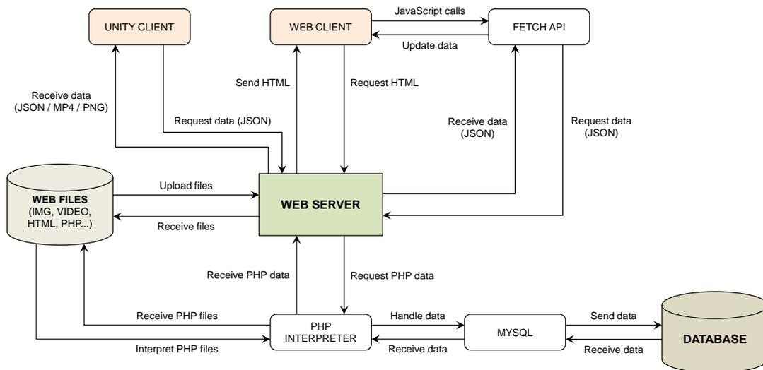
**Figure 7:** Client-server architecture of the TAECon platform.
