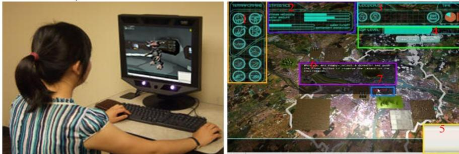
**Figure 8.** The left image shows the eye tracking set up, the right a screen shot of the game's terraforming simulation. The colored rectangles indicate predefined areas of interest (AOI) for gaze data analyses.
