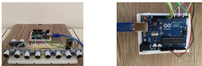
Figure 5. The sonar system was tested on the board before final installation (left), and using a USB port to program Arduino (right).
